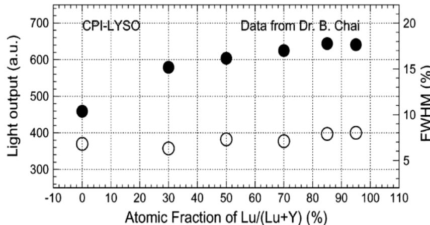
The light output (solid dots, left scale) and the energy resolution (open dots, right scale) as a function of the lutetium fraction in LYSO
